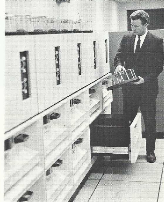
All information put into SENTRY is retained on magnetic tape discs which hold some 60,000,000 words of information.
