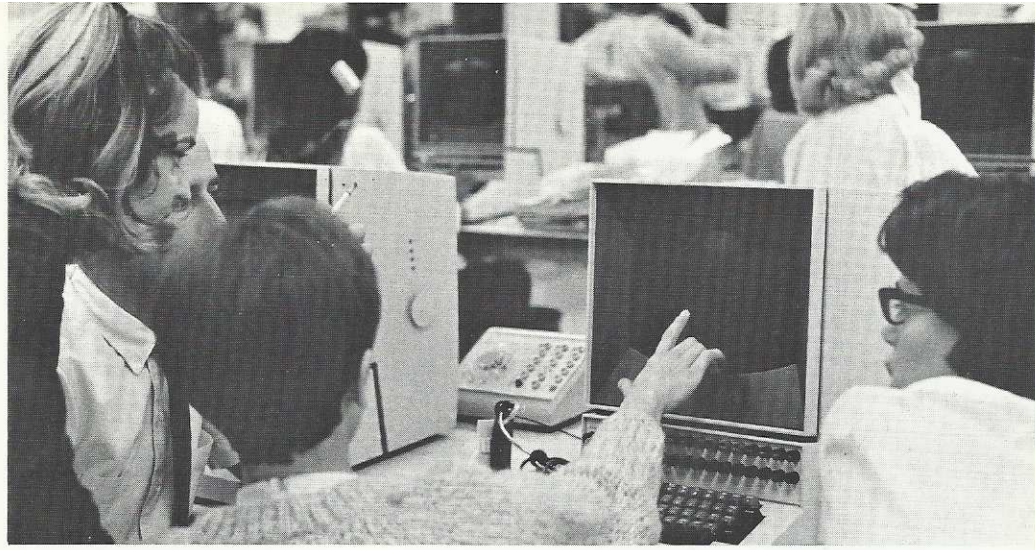
Cathode ray tube agent sets which appear to be typewriters with television-like screens make up a portion of the highly complex SENTRY system. 181 television-like sets are located throughout Frontier's system, with 101 being concentrated in Denver.
