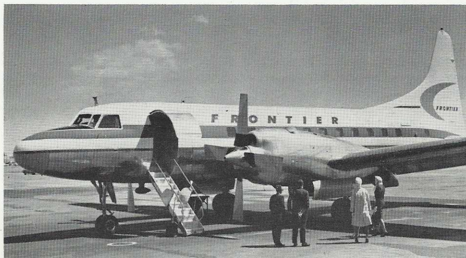
SQUARE-TIPPED, FOUR-BLADED PROPELLERS and the big nacelles enclosing the turbine Allison engines distinguish the Convair 580 jet prop aircraft. The new color scheme consists of a band of turquoise in the mid-section of the fuselage with a thinner band of gold dividing the painted and unpainted sections and is completed by a gold crescent featured on the high vertical stabilizer with the addition of "Frontier" being incorporated in the design. Both the exterior and interior of the aircraft was designed by A. Baker Barnhart of New York City.
