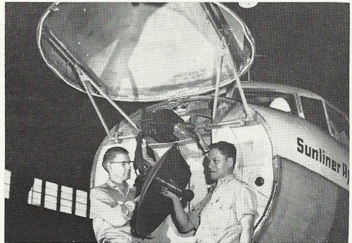
Weather radar antenna in the nose of a "Radar Convair" gets a check from Chuck Carter and Sylvester Cuellar, radio mechanics.
