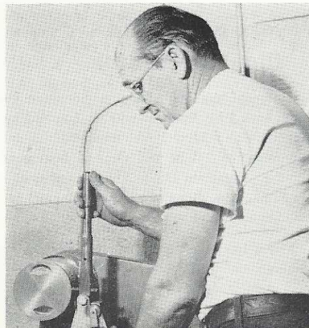
ONE . . . Bill Long, Denver maintenance, is working on one of several ideas which earned him prize money for the best suggestions of the month. This tool is in use in the engine Shop and is for removing carbon from piston ring grooves.
