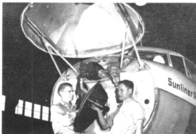
Weather radar antenna in the nose of a "Radar Convair" gets a check from Chuck Carter and Sylvester Cuellar, radio mechanics.
