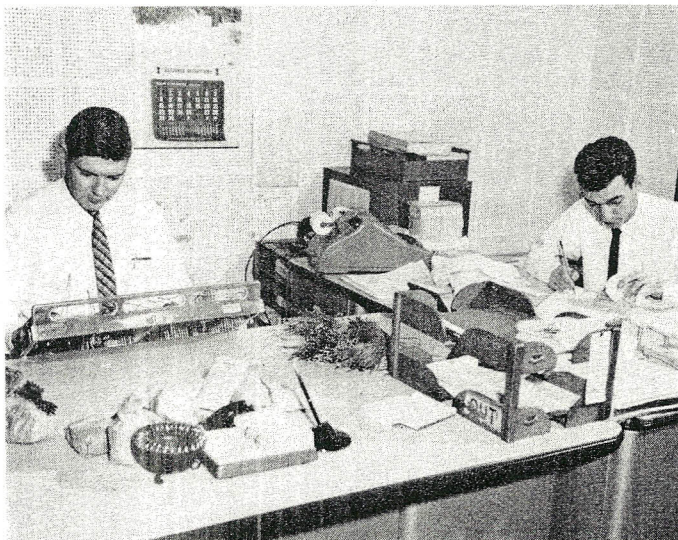
Chuck Turner, Manager of the Machine Accounting Department, wires up a tabulator control panel. This is the electric brain which triggers each punched card for information totals. Vern Korn, Senior Tab Operator, checks all outgoing work to correct possible discrepancies before the material is released.
